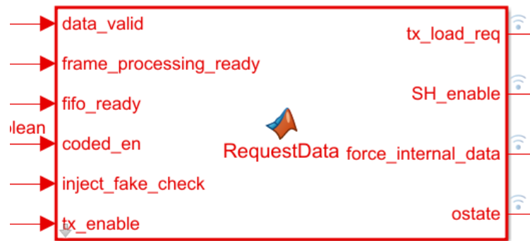
Fig. 4.5 Finite state machine for requesting data from software or internal data generator
